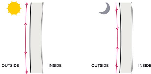
If the hooks on the multipoint lock are not thrown throughout the day and the centre keep setting is too tight, the top and bottom of the door will be in unsupported tension and will eventually stand proud of the inner face of the profile. This will make the hooks on the lock become stiff, as they cannot draw themselves into the hook keep.
