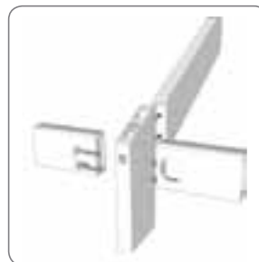
Eaves purlin - exploded view
